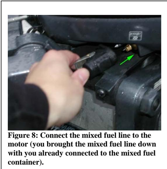
**Figure 8: Connect the mixed fuel line to the motor (you brought the mixed fuel line down with you already connected to the mixed fuel container).**
