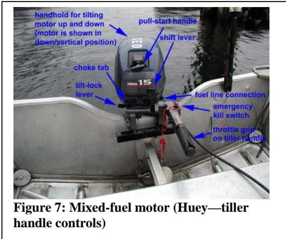
**Figure 7: Mixed-fuel motor (Huey—tiller handle controls)**
