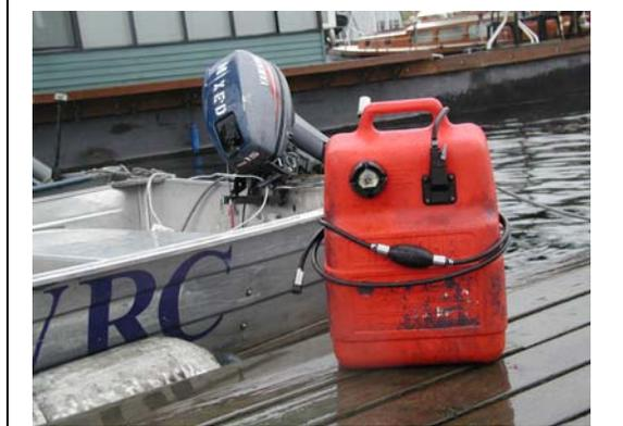
**Figure 2: Metal launches use mixed fuel.**
